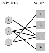
Fig. 6. A bipartite graph indicating which capsules can be placed on which nodes.
