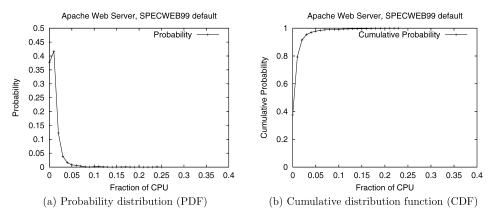
Fig. 3. Profile of the Apache Web server using the default SPECWeb99 configuration.
