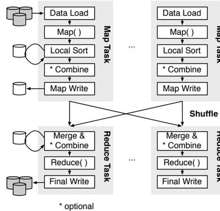
Fig. 1. Architecture of the Hadoop implementation of MapReduce.
