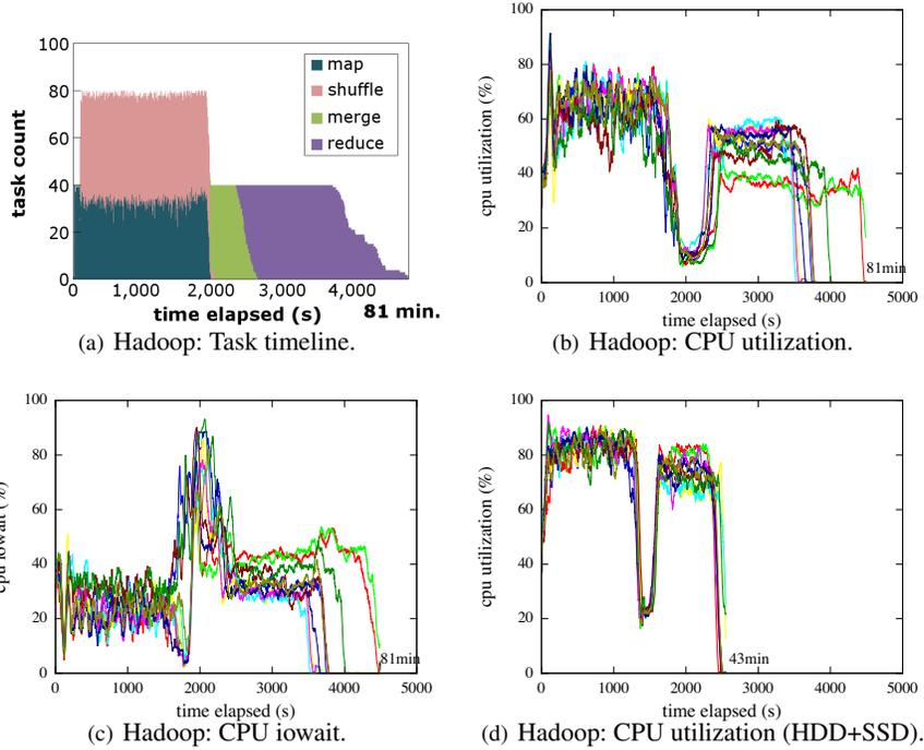
Fig. 2. Experimental results using the sessionization workload.
