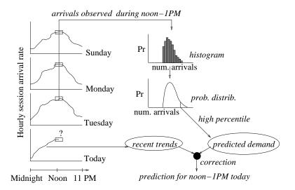
Fig. 4. The workload prediction algorithm.
