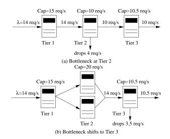
Fig. 1. Strawman approaches for provisioning a multi-tier application.
