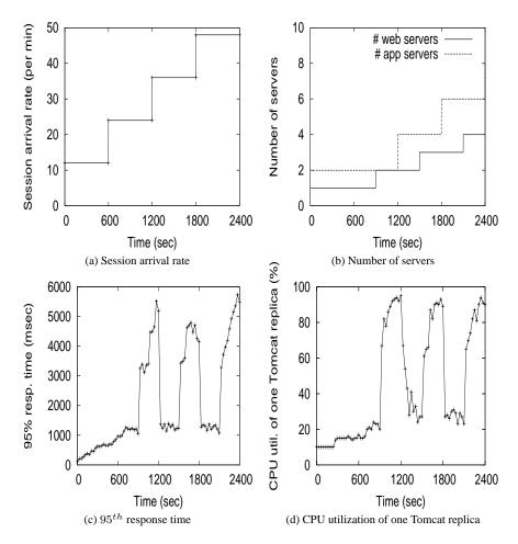
Fig. 7. Rubbos: Independent per-tier provisioning.
