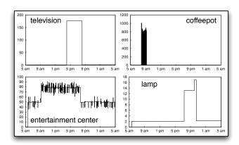
Figure 3. Power data for example interactive loads. Occupant behavior, which is not readily predictable, determines when these loads draw power.
