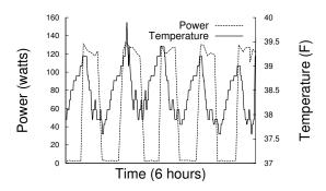
Figure 5. A depiction of slack in our refrigerator's simple on-off control loop. The compressor turns on once the internal temperature reaches an upper threshold, and turns off once it reaches a lower threshold.
