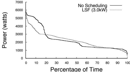
Figure 9. Load duration curves for a typical summer day with and without scheduling when using an electric vehicle.
