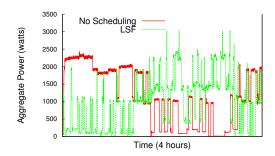
Figure 10. Power usage with and without LSF scheduling using using our smart home testbed with real background loads over a 4-hour period.
