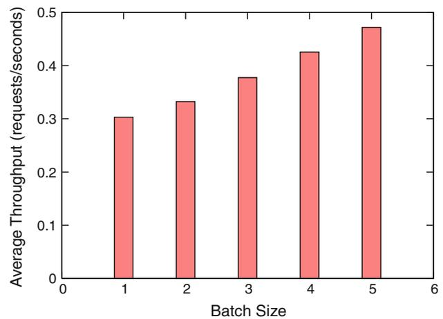
**Fig. 15** AFQ shows better global performance in terms of average throughput in requests/s as batch size increases. For this experiment, each increment in the batch size results in roughly a 10% improvement
