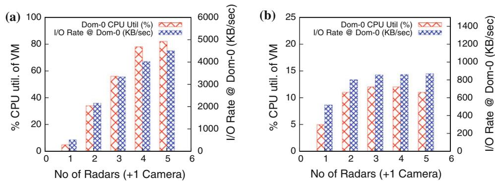
**Fig. 9** Utilization of Domain-0's 40 % CPU share and I/O rate for radars with and without actuation costs. The number of vsensors vary from 1 to 5, where the first vsensor is a PTZ camera and the remaining vsensors are radars. **a** No actuation costs and **b** includes actuation costs
