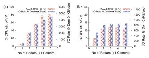
Fig. 9 Utilization of Domain-0's 40 % CPU share and I/O rate for radars with and without actuation costs. The number of vsensors vary from 1 to 5, where the first vsensor is a PTZ camera and the remaining vsensors are radars. **a** No actuation costs and **b** includes actuation costs
