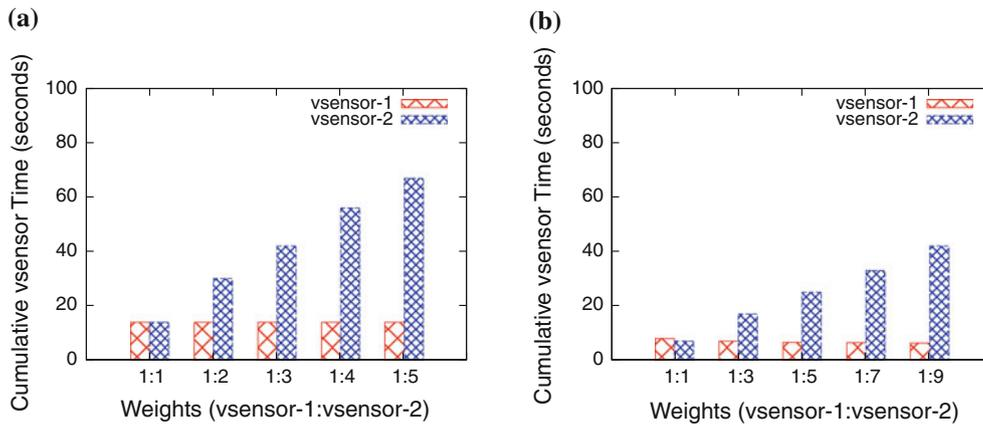
**Fig. 12** AFQ enforces performance isolation over large numbers of requests. The ratio of the total vsensor time for the two continuous scan workloads is in proportion to the assigned weights. **a** Camera and **b** radar
