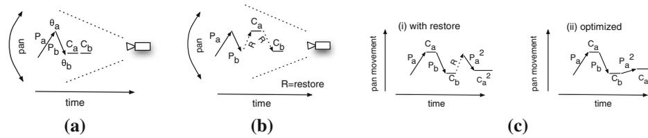
**Fig. 1** Examples showing why request interleaving is challenging for steerable sensors. **a** Naive interleaving  $P_a P_b C_a C_b$  yields incorrect results, **b** correct interleaving  $P_a P_b C_a C_b$  with state restorations and **c** optimizing state restoration costs
