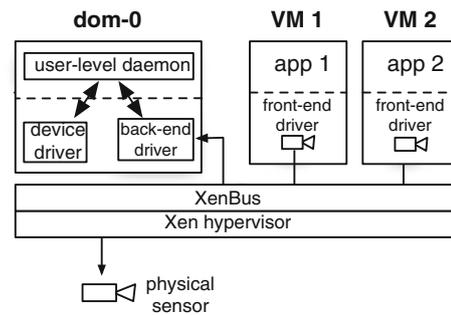
**Fig. 5** MultiSense uses Xen's split-driver framework for communication, and a user-level daemon in Domain-0 to maintain vsensor VSMs and execute scheduling policies. Each request passes from application → front-end driver → back-end driver → daemon → device
