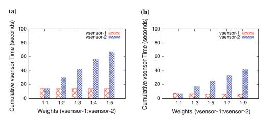
Fig. 12 AFQ enforces performance isolation over large numbers of requests. The ratio of the total vsensor time for the two continuous scan workloads is in proportion to the assigned weights. a Camera and b radar
