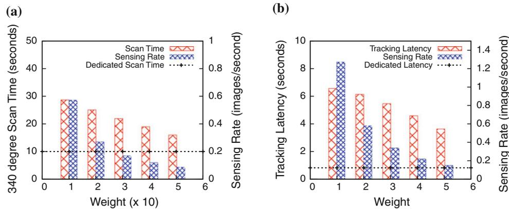
**Fig. 20** For the camera, MultiSense is able to serve concurrent sensing applications. A continuous monitoring application (a) and an object tracking application (b) both maintain tolerable performance
