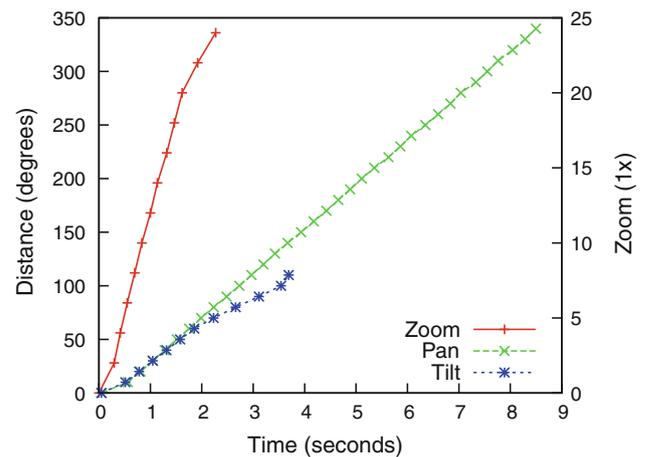
**Fig. 6** Time benchmarks for the pan, tilt, and zoom actuators of sony SNC-SRZ30N network camera that show the distance moved by the actuator is roughly linear to the time and energy required to complete the actuation
