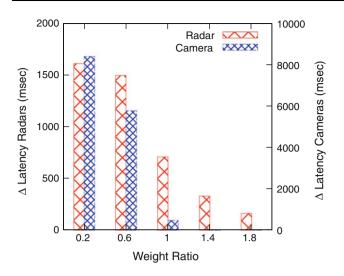
Fig. 22 The difference in latency when coordinating multiple vsensors on different nodes to sense the same point
