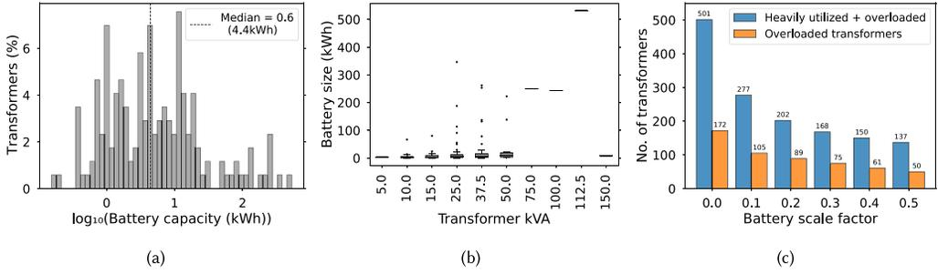
Fig. 14. (14(a)) Energy storage capacity required to limit utilization to no more than 125% across all transformers, and (14(b)) distribution of energy storage capacity needed to limit overloading based on transformer capacities, and (14(c)) reduction in number of overloaded and heavily utilized transformers with increasing battery scale factor.
