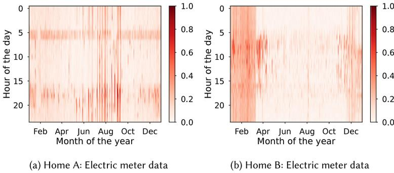
Fig. 6. (6(a)) Normalized energy consumption for an individual home with alternate heating energy source, e.g., gas (Home A), and (6(b)) normalized energy consumption for another home using electric heating (Home B).
