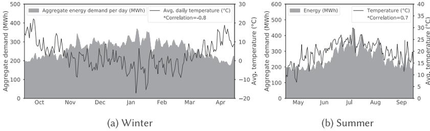
Fig. 3. Variations in daily aggregated electricity consumption at the grid level for the entire year.
