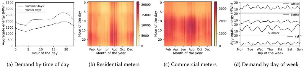
Fig. 2. (2(a)) Aggregate power consumption by time of day for all meters, and (2(b)) aggregate electricity consumption for all residential buildings across the year, and (2(c)) aggregate electricity consumption for all commercial buildings, and (2(d)), aggregate demand at the grid level for a representative week in each season.
