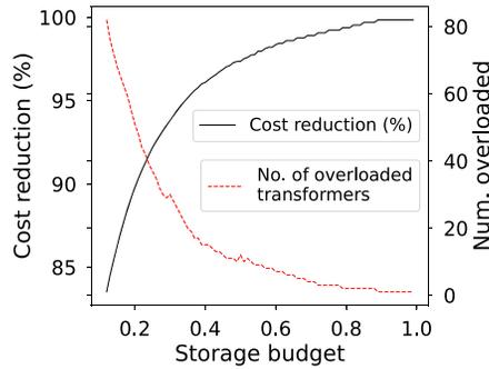
Fig. 15. Tradeoff between the number of overloaded transformers and net value gain under budgetary constraints.
