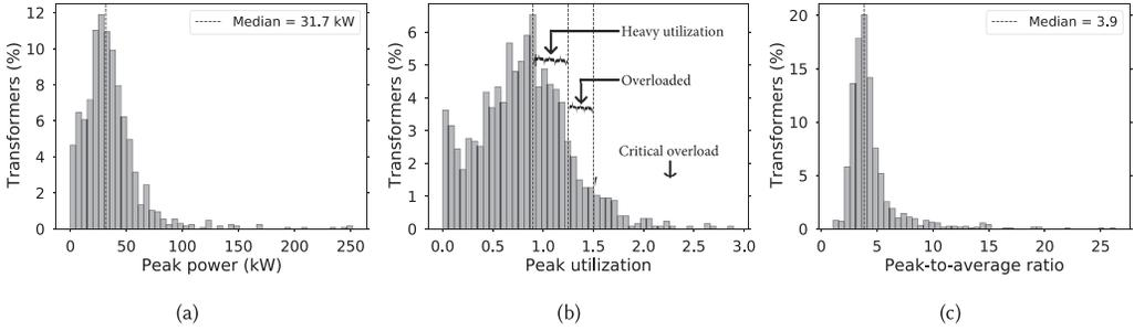
Fig. 11. (11(a)) Distribution of absolute power demand over a year, and (11(b)) distribution of transformer overloading over a year, based on the peak utilization, and (11(c)) distribution of transformer peak-to-average ratio over the year.
