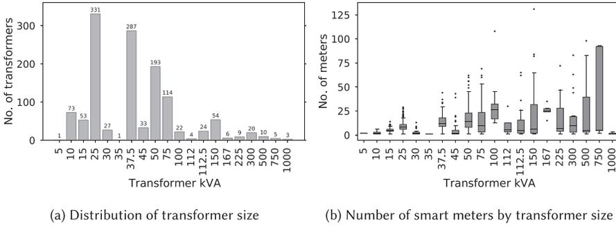
Fig. 1. (1(a)) Distribution of transformers by capacity, and (1(b)) Distribution of smart meters connected to transformers of varying capacity.
