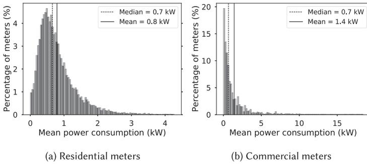
Fig. 5. (5(a)) Distribution of average power consumption per home, (5(b)) Distribution of average power consumption by commercial meters.
