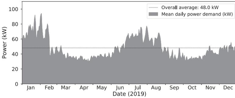
Fig. 9. Graph illustrating the load on a sample transformer over a year with demand peaking during winter and summer seasons.
