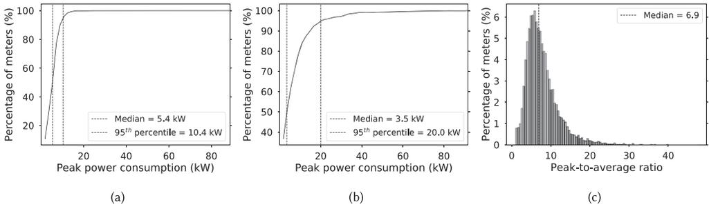
Fig. 8. (8(a)) Cumulative distribution function of absolute peak power usage by residential meters, and (8(b)) cumulative distribution function of absolute peak power usage by commercial meters, and (8(c)) distribution of power peak-to-average ratio over the year for all meters.
