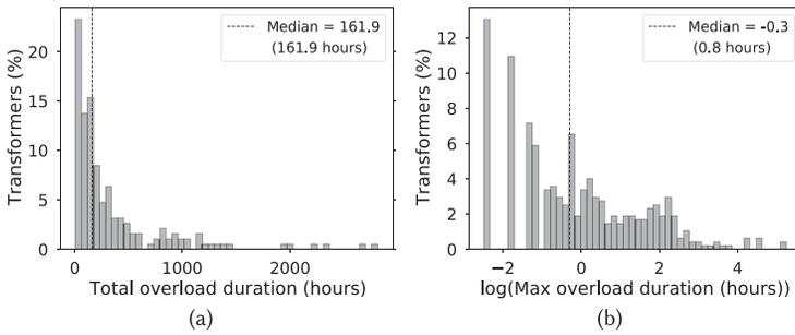
Fig. 12. (12(a)) Distribution of the total number of hours during which transformers were overloaded during the year, and (12(b)) distribution of the maximum sustained period of overloading (log scale).
