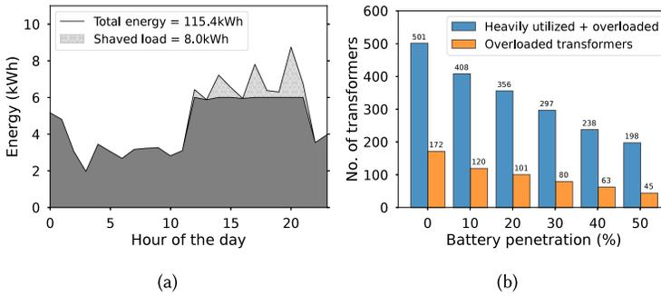
Fig. 13. (13(a)) Original and shaved load for a sample home with an installed battery during a particular day, and (13(b)) reduction in number of heavily utilized and overloaded transformers with increase in home battery penetration.
