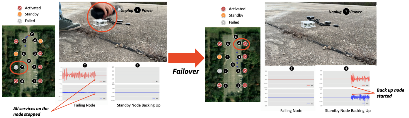
Fig. 8: Illustration of a node failure and its corresponding failover process. The battery is unplugged from node 7, which deactivates the entire node, causing a node failure. Standby node four is then activated to replace node 7.
