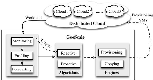
**Figure 1: GeoScale Design and Basic Operation.**
