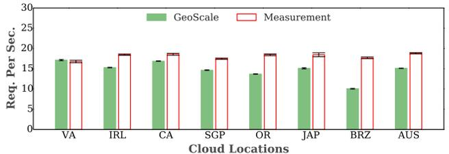
**Figure 2:** Comparisons of GeoScale’s capacity modeling with empirical measurement for small server instances.
