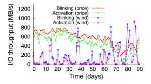
Figure 6: The maximum aggregate I/O throughput for blinking is greater than for activation for both our wind energy and variable price scenarios.
