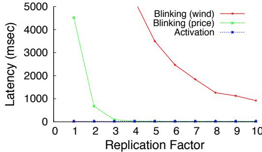
**Figure 7: A small amount of replication is capable of significantly improving data access latency with blinking.**
