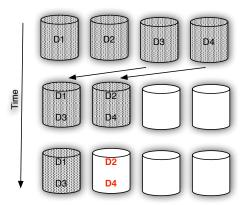
Figure 2: Power variations may cause the subset of active servers storing a data set's primary replicas to decrease, which triggers costly migrations to keep data accessible. At low power levels, some data is certain to be inaccessible.
