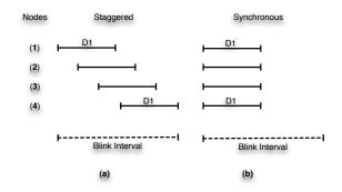
Figure 3: Power variations decrease the fraction of time each server is active during a blink interval. No migrations are necessary to adjust to power variations, since all blocks are accessible for a fraction of each blink interval.
