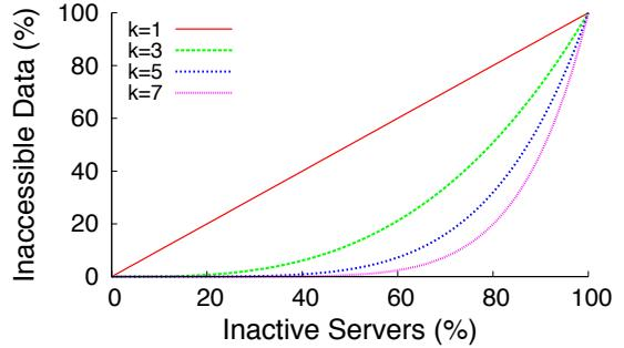
**Figure 1: Inactive servers result in inaccessible data. Replication mitigates, but does not eliminate, the problem, especially for high percentages (>50%) of inactive servers.**
