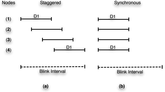
**Figure 4: A staggered server blinking pattern is able to use replication to maximize the availability of data and decrease average I/O latency as power varies.**
