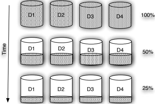
**Figure 3: Power variations decrease the fraction of time each server is active during a blink interval. No migrations are necessary to adjust to power variations, since all blocks are accessible for a fraction of each blink interval.**
