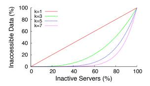
Figure 1: Inactive servers result in inaccessible data. Replication mitigates, but does not eliminate, the problem, especially for high percentages (>50%) of inactive servers.
