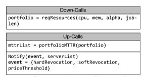
Fig. 5. ExoSphere's design architecture. The job managers for each application implement the resource allocation requests and the fault tolerance policies.
