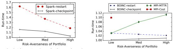
Fig. 9. Spark job run-time (normalized to on-demand servers) when one market fails.
