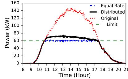
Figure 13: Maintaining the limit at a 1-minute interval.
