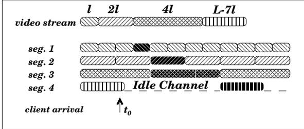
Figure 3: GDB segmenting scheme for Periodic Broadcast
