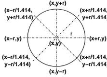
Figure 7: Potential neighbors to place access points to extend coverage.
