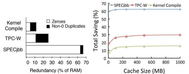
Fig. 13. (a) Each application has different levels of redundancy, in some cases mostly from empty zero pages. (b) Increasing the cache size leads to diminishing returns; we use a 100-MB cache in our remaining experiments.
