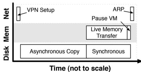
Fig. 4. Phases of a migration for nonshared disk, memory, and the network in CloudNet.
