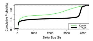
Fig. 6. During a kernel compile, many pages only experience very small modifications. TPC-W has some pages with small modifications, but more than half are almost completely changed.
