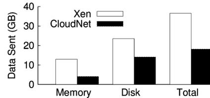
Fig. 16. CloudNet saves nearly 20 GB of bandwidth when simultaneously migrating four VMs.
