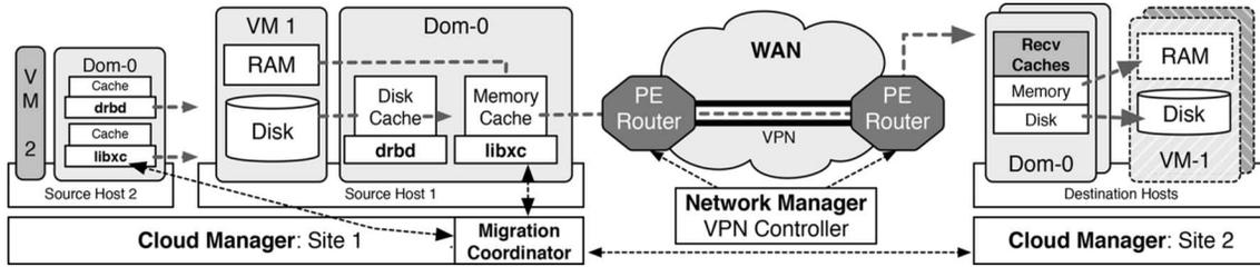
Fig. 8. After the VPN Controller establishes connectivity, the Cloud Manager's Migration Coordinator initiates each transfer. CloudNet uses separate caches for each memory and disk migration.
