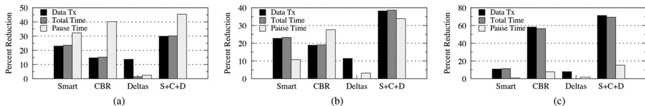
Fig. 11. CloudNet's optimizations affect different classes of application differently depending on the nature of their memory accesses. Combining all optimizations greatly reduces bandwidth consumption and time for all applications. (a) Kernel Compile. (b) TPC-W. (c) SPECjbb.
