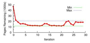
Fig. 7. Number of pages to be sent quickly levels off. Intelligently deciding when to stop a migration eliminates wasteful transfers and can lower pause time.
