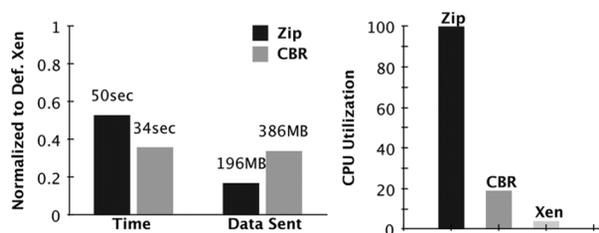
Fig. 18. Zip compression significantly reduces the data size, but has a very high computation cost.
