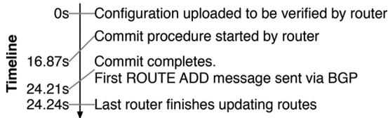
Fig. 9. Timeline of operations to add a new endpoint.
