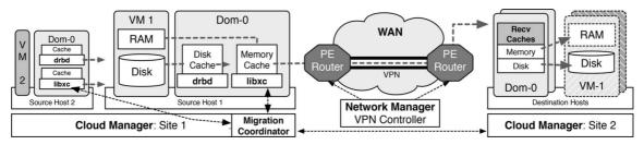
Fig. 8. After the VPN Controller establishes connectivity, the Cloud Manager's Migration Coordinator initiates each transfer. CloudNet uses separate caches for each memory and disk migration.
