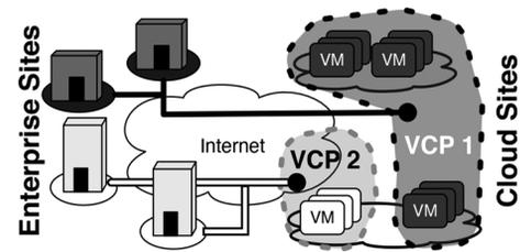
Fig. 1. Two VCPs isolate resources within the cloud sites and securely link them to the enterprise networks.
