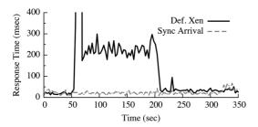
Fig. 17. If a multitier migration is not synchronized, performance can suffer badly.
