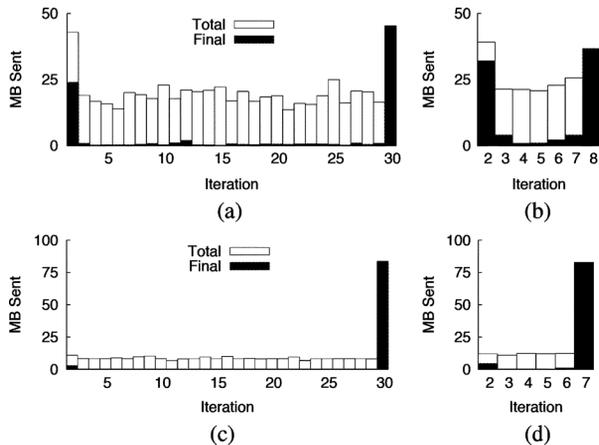
Fig. 12. Smart Stop reduces the iterations in a migration, significantly lowering the number of “useless” page transfers that otherwise are repeated. (a) TPC-W Default Xen. (b) TPC-W Smart. (c) SPECjbb Default Xen. (d) SPECjbb Smart.
