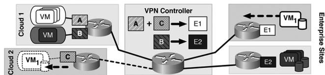
Fig. 3. VPN Controller remaps the route targets (A, B, C) advertised by each cloud data center to match the proper enterprise VPN (E1 or E2). To migrate VM<sub>1</sub> to Cloud Site 2, the VPN controller redefines E1's VPN to include route target A and C, then performs the disk and memory migration.
