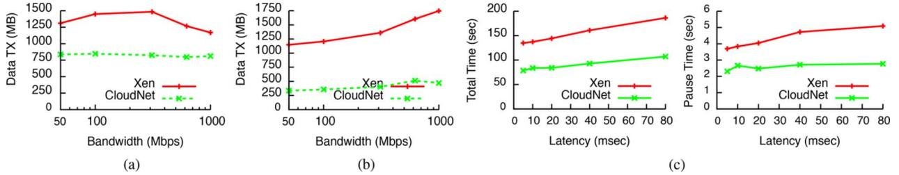
Fig. 15. (a) TPC-W bandwidth usage and (b) SPECjbb bandwidth usage. CloudNet's optimizations significantly reduce bandwidth consumption. (c) TPC-W latency impact. Increased latency has only a minor impact on the migration process, but may impact application performance due to synchronous disk replication.
