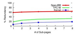
Fig. 5. Each application has a different level of redundancy. Using finer granularity finds more redundancy, but has diminishing returns.
