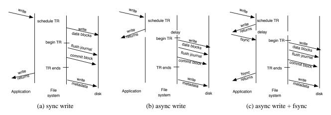
Figure 4: Event sequence for a synchronous write, an asynchronous write, and asynchronous write followed by a fsync.
