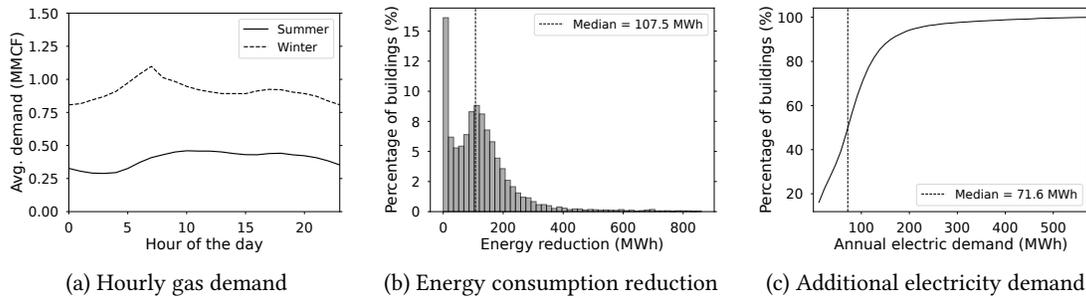
**Figure 10: Distribution of (a) average gas load demand by time of day after transitioning to electric heat pumps, (b) energy consumption reduction across buildings after transition to electric heat pumps, and (c) additional electric demand exerted on the system after transitioning from gas to electric heat pumps (cumulative).**
