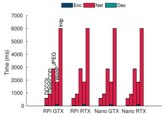
Figure 7: End-to-end offloading latency using LTE
