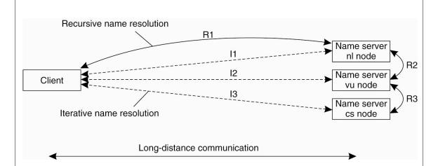
Comparison between recursive and iterative name resolution with respect to communication costs.
