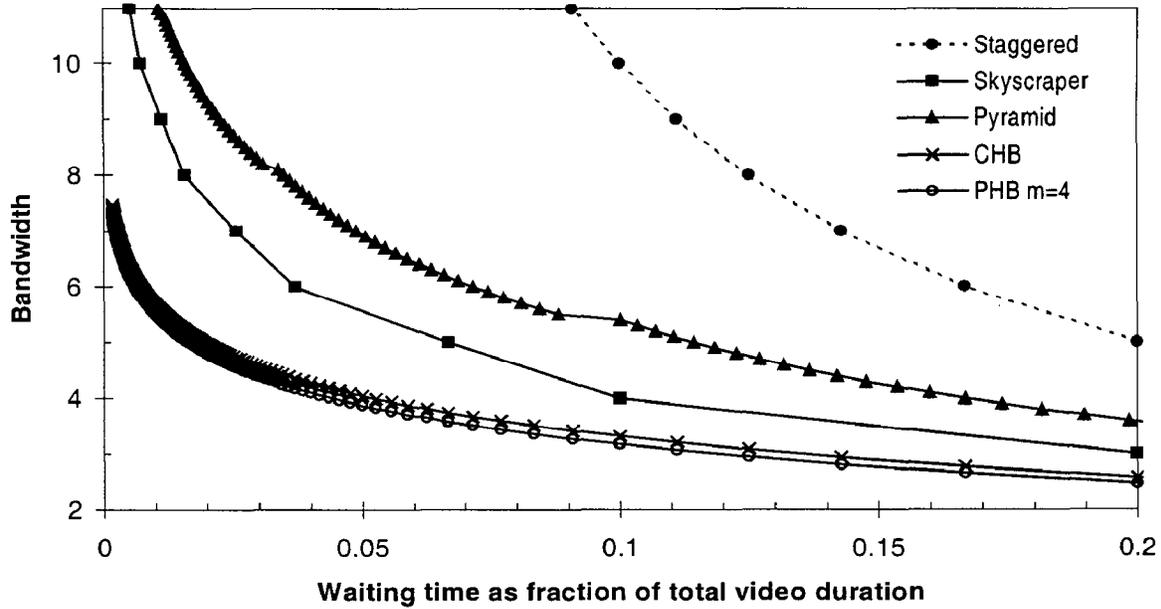
Figure 2: Bandwidth requirements of typical broadcasting protocols
