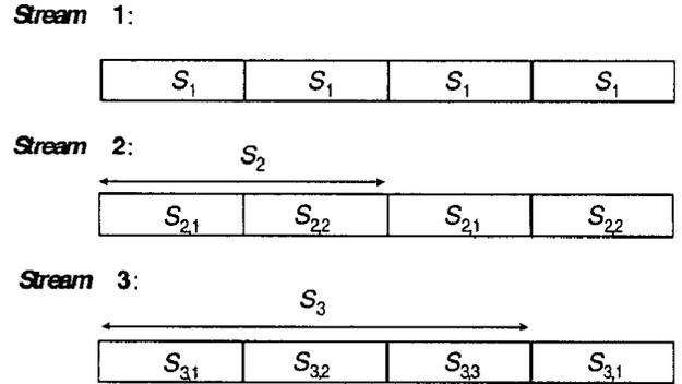
Figure 1: An illustration of the first three segments of a video under harmonic broadcasting
