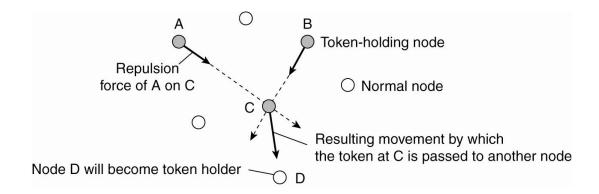
Moving tokens in a two-dimensional space using repulsion forces.
