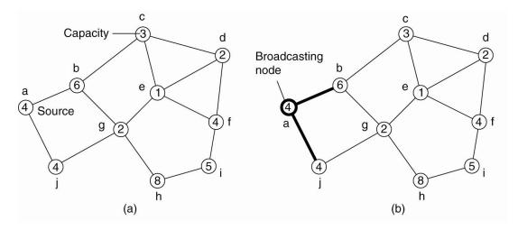
• Election algorithm in a wireless network, with node a as the source. (a) Initial network. (b)–(e) The build-tree phase
