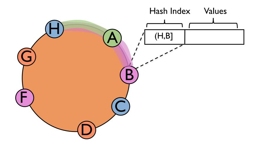
Node additions, failures require transfer of key-ranges
