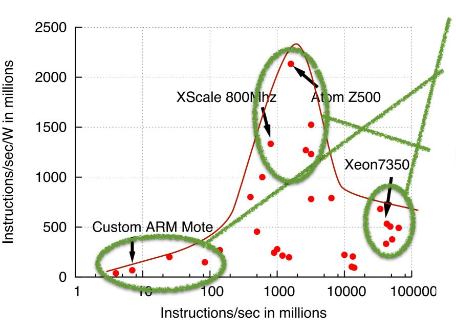
Fastest processors exhibit superlinear power usage
