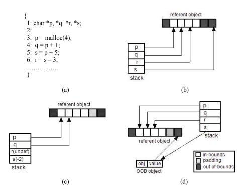
Figure 1. (a) Simple C program, memory states of (b) uninstrumented execution, (c) instrumentation with Jones and Kelly Checker, (d) instrumentation with CRED.
