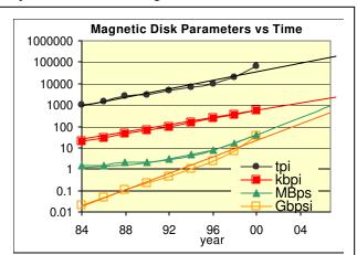
**Figure 1**: Disk capacity has improved 1,000 fold in the last 15 years, consistent with Moore's law, but the transfer rate MBps has improved only 40x in the same time. The metrics are tracks per inch (tpi), thousands of bits per linear inch of track (kbpi), megabits per second as the media spins (MBps), and gigabits per square inch
