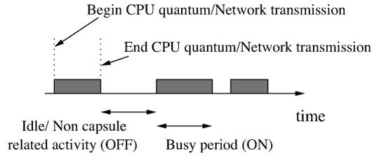
Fig. 1. An example of an On-Off trace.
