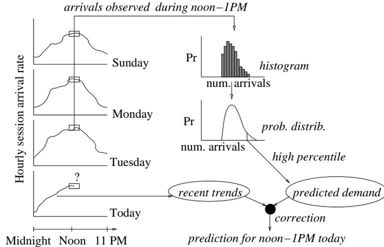
Fig. 4. The workload prediction algorithm.
