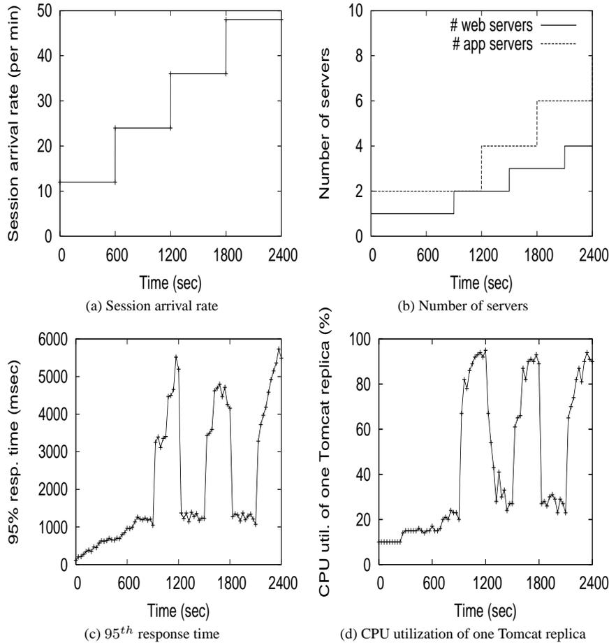
Fig. 7. Rubbos: Independent per-tier provisioning.
