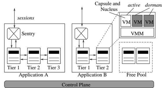
Fig. 3. Hosting Platform Architecture.
