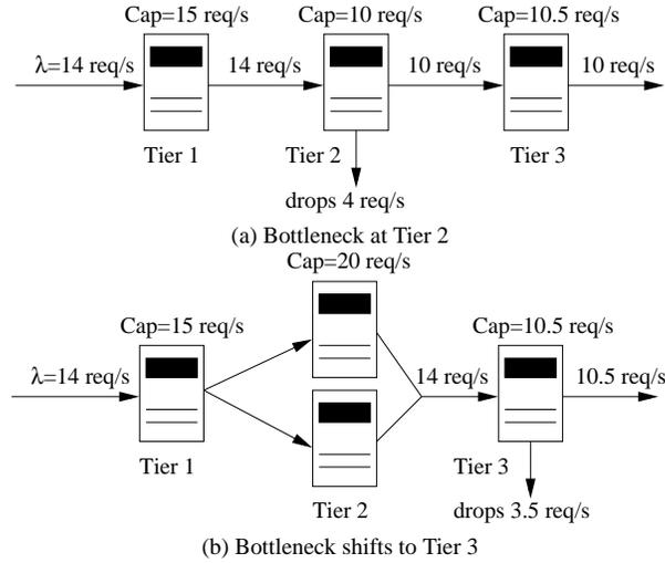
Fig. 1. Strawman approaches for provisioning a multi-tier application.
