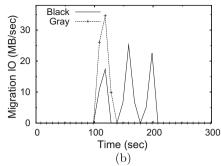
Fig. 8. The gray-box system balances the system more quickly due to more informed decision making. The black-box system must perform migrations sequentially and incurs an additional migration.
