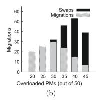
**Fig. 11.** (a) Using time-series predictions (the dotted lines) allows Sandpiper to better select migration destinations, improving stability. (b) Higher levels of overload requires more migrations until there is no feasible solution.
