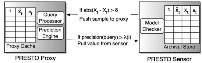
Fig. 2. The PRESTO proxy comprises a prediction engine, query processor and a cache of predicted and real sensor values. The PRESTO sensor comprises a model checker and an archive of past samples with the model predictions.
