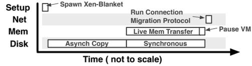
Figure 5: The phases of a migration for non-shared disk, memory and the network in VMShadow.
