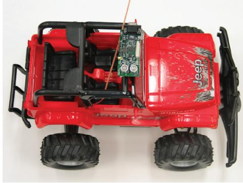
Fig. 14. Remote control toy car with a Cricket node on the top.
