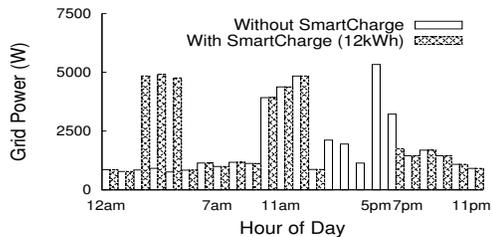
**Figure 4: Example from January 3rd with and without SmartCharge using Illinois prices from Figure 3.**
