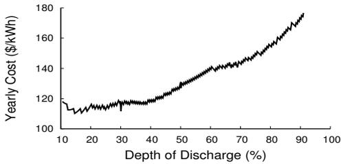
**Figure 13: Amortized cost per kWh as a function of depth of discharge.**
