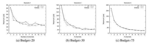
Figure 5: Effect of varying the number of channels at each location.
