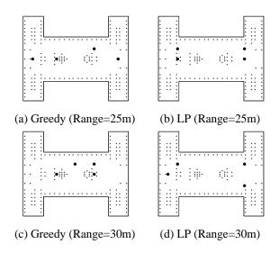
Figure 6: Access Point placement in CS Bldg.
