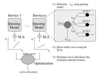
Figure 4: Dynamic provisioning in the control plane.
