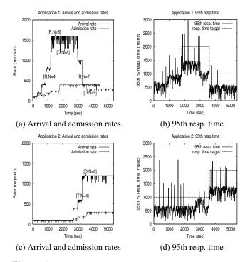
**Figure 6**: Dynamic provisioning and admission control: Performance of Applications 1 and 2. D: Default invocation of provisioning, T: Provisioning triggered by excessive drops, [N=n]: size of the server set is n now. Only selected provisioning events are shown.
