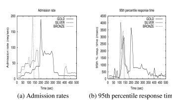
**Figure 8**: Performance of the threshold-based admission control. At t=135sec, the threshold was set to reject all Bronze requests; at t=180sec, it was updated to reject all Bronze and Silver requests; at t=210sec it was updated to also reject Gold requests with a probability 0.5; finally, at t=390sec, it was again set to reject only Bronze requests.
