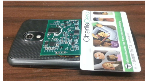
Figure 10: Our EnGarde prototype meets the form factor needs required for semi-permanent attachment to a mobile phone. Here, we show it on the back of a Galaxy Nexus
